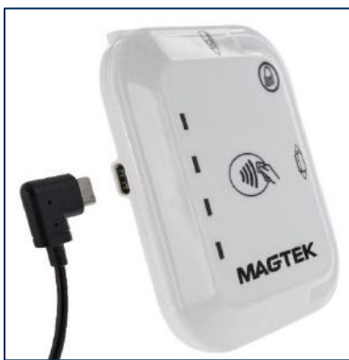
Figure 2-1 - Connecting tDynamo to a Host via USB
